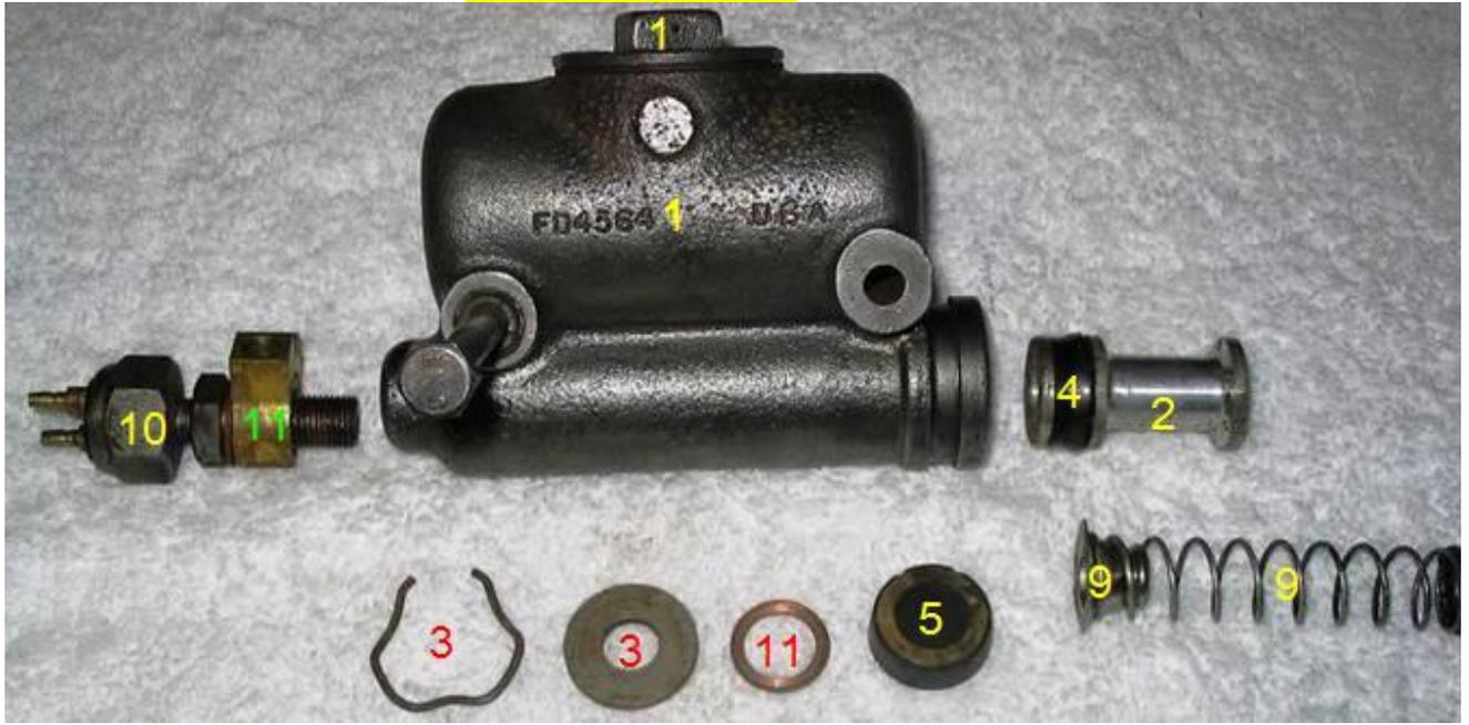
The master cylinder is made up of the following parts:
