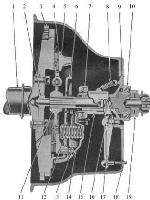
FIG. 21 -- CLUTCH ASSEMBLY
