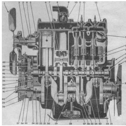
FIG. 2 -- SIDE SECTIONAL VIEW OF ENGINE
