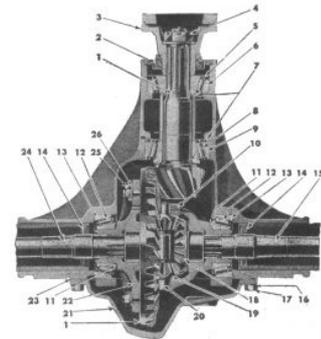
FIG. 26 -- FRONT AXLE DIFFERENTIAL
