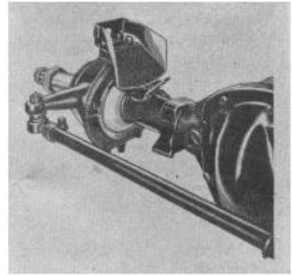
FIG. 5 -- KNUCKLE OIL SEAL
