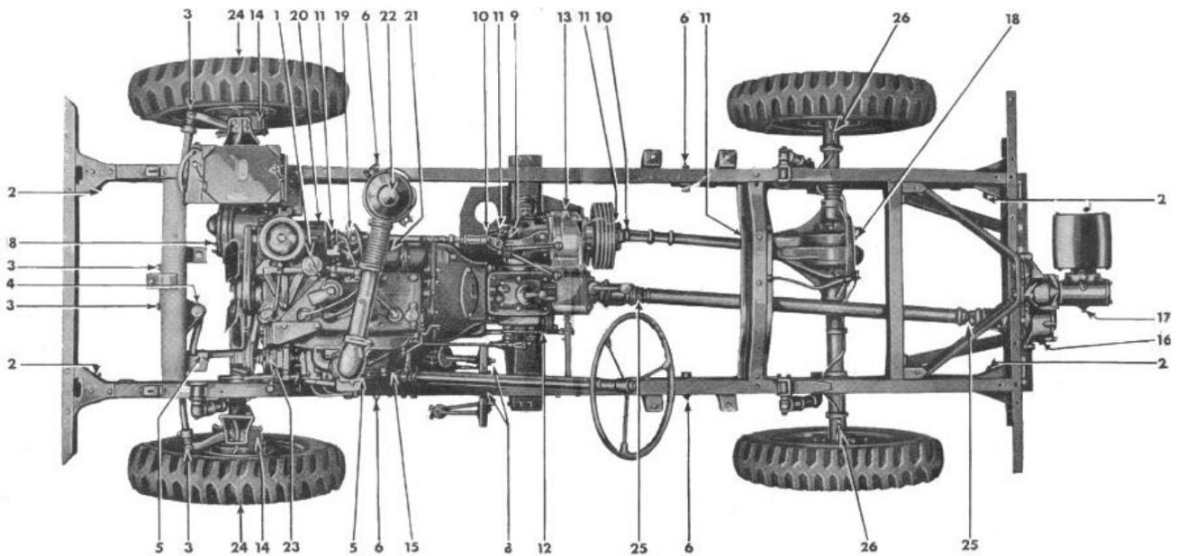
FIG. 17 -- CHASSIS, SHOWING PARTS REQUIRING LUBRICATION
