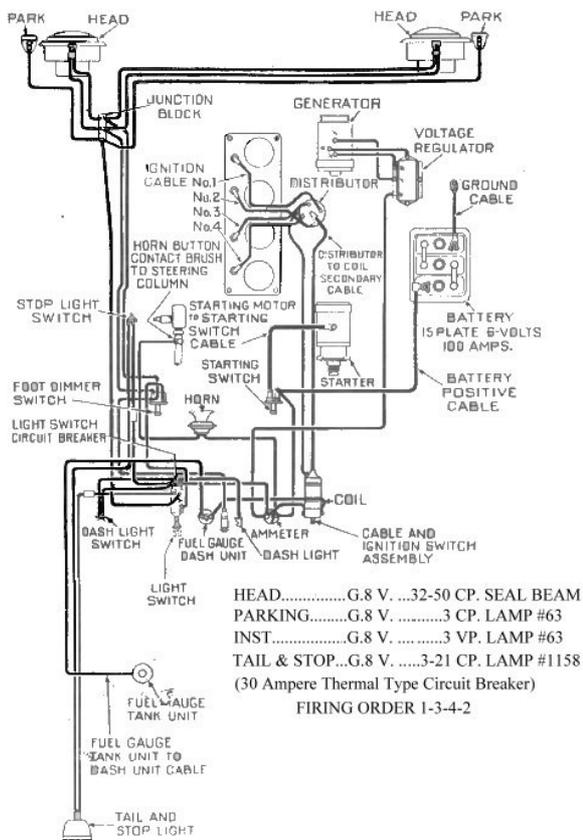
FIG. 16 -- WIRING DIAGRAM
